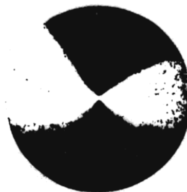
Figure 3. Nineteenth century students of pleochroism frequently referred to their observation of absorption brushes shown here in tourmaline. A highly absorbing, anisotropic crystal viewed with the eye close to the surface along the optic axis reveals on a colored ground, two dark hyperbolic brushes. These come about in some crystals when absorption differs markedly for rays propagating along or obliquely to the optic axis. 119 (Reprinted with permission from ref 119. Copyright 1960 Consultants Bureau.)
