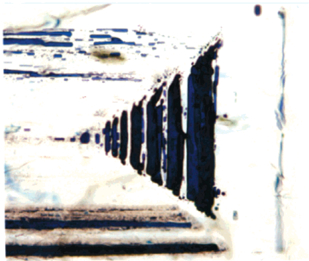
Figure 12. Lead acetate trihydrate crystals containing methylene blue in solution inclusions confined to the \{100\} growth sector. View along [010] . Horizontal dimension = 9 mm.
